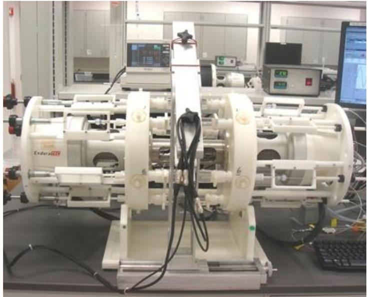
**Stent Graft Tester Adapted for Percutaneous Heart Valve Testing**
