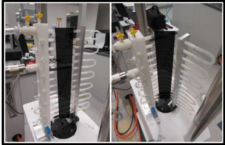
*Figure 3- MDT Bend/Wag testing of peripheral stents.*
