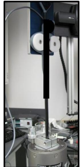
*Figure 2- MDT Torque-to-Fracture testing of an aortic leaflet repair device.*
