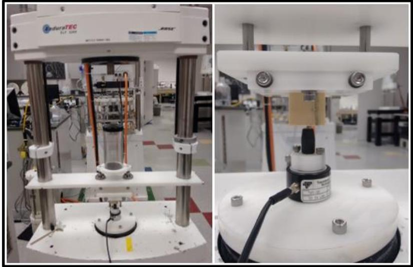
*Figure 1-MDT Bone Screw Insertion & Removal Torque Testing.*
