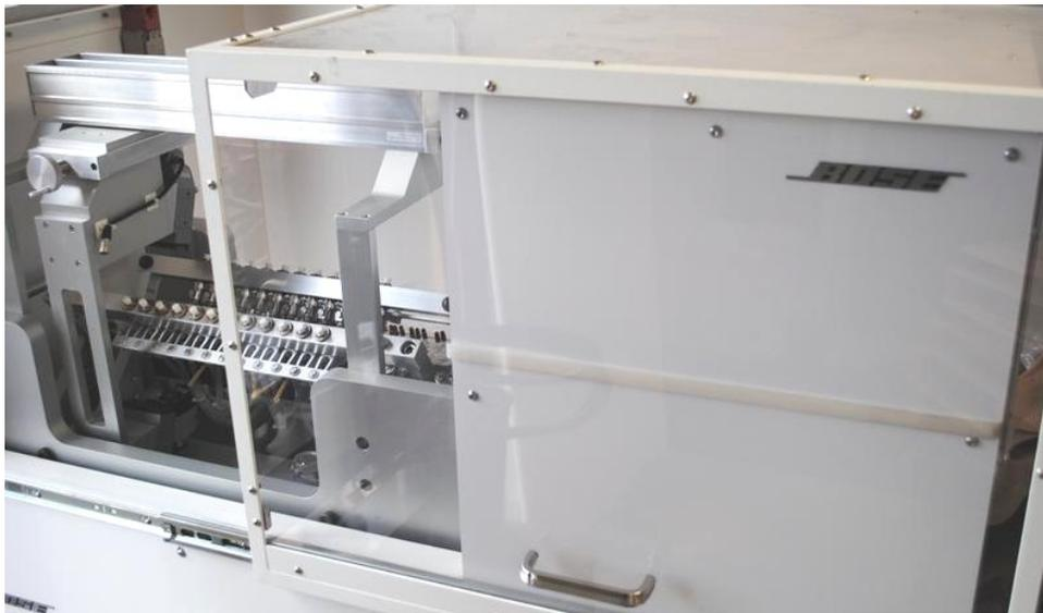
**Figure 2: Bose ElectroForce 9500 system (12-stations)**
