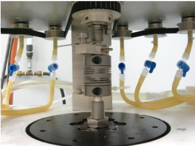
**Figure 6: System of pulleys that rotate each sample**
