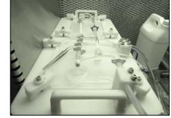
For simulated use testing, the device and deployment system are tracked through an in vitro model simulating the vascular anatomy (shown above), and then the device, a stent in this case, is deployed with a balloon catheter into a mock vessel. The flow loop is maintained at a pre-specified flow rate for several minutes, and new mock vessels are used for each test repeat.
