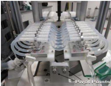
Peripheral Stent Pure Bending Fixture
