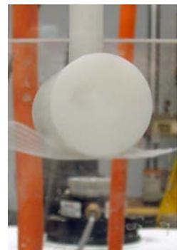
worst-case loading conditions may be simulated by clamping the device at the extreme ends and loading at the half point.
