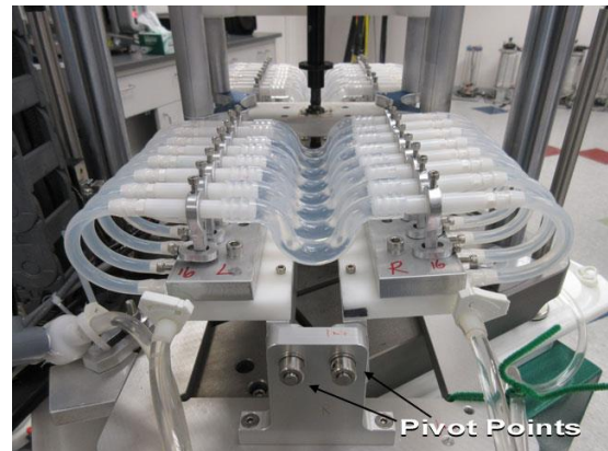
Pure Bending Fixture for Peripheral Stents
