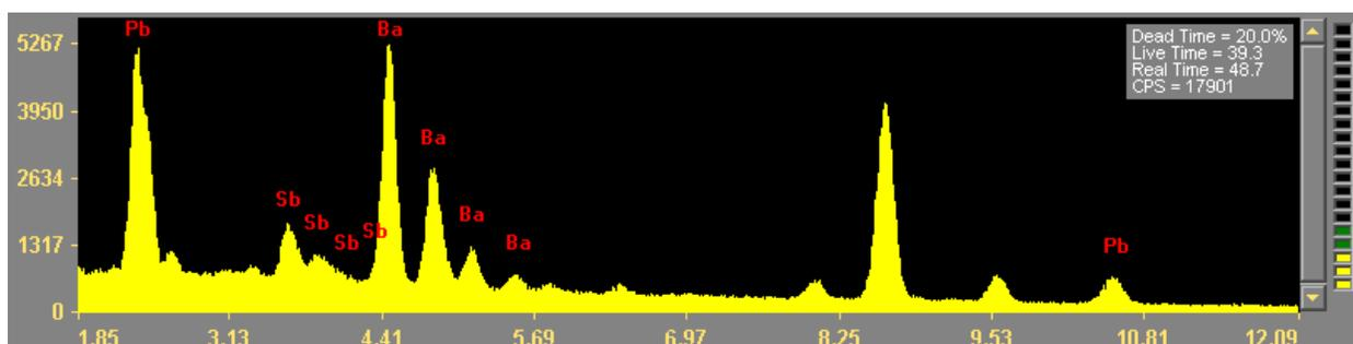
Figure 4: EDS Compositional Spectrum
