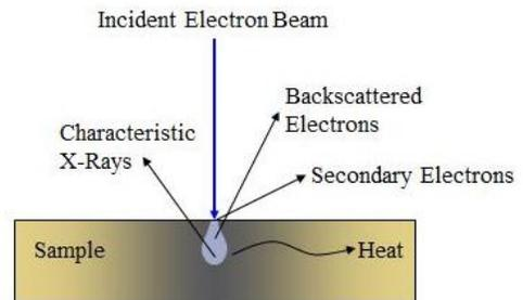
Figure 1: Electron Beam Interactions
